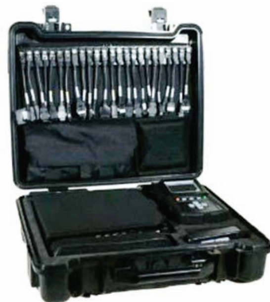
The Cellebrite Law Enforcement Kit contains adaptors for several dozen types of cell phones.
